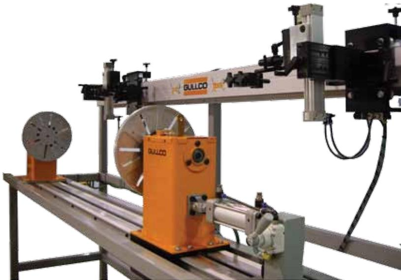
Automate your circumferential welding operations, add efficiency and increased precision with the highly versatile Automatic Rotary Weld System
